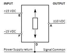
A through F: Connector pin assignments
