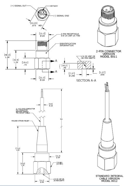
All values are typical at +24°C, 100Hz and 15Vdc excitation unless otherwise stated. Measurement Specialties reserves the right to update and change these specifications without notice. Standard product parameters are described in PSC-1003 for Plug & Play AC Accelerometers.
