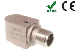
**The Model 8021-01 & 8022-01** are internally shielded rugged IEPE accelerometers designed for harsh environments. The accelerometers are available in ±10g, ±80g & ±500g dynamic ranges and have a flat bandwidth up to greater than 12kHz. The model 8021-01 features a side exit MIL-C-5015 connector while the model 8022-01 features an integral cable. The units are hermetically sealed and are designed to operating in temperature ranges from -55°C to +125°C.
