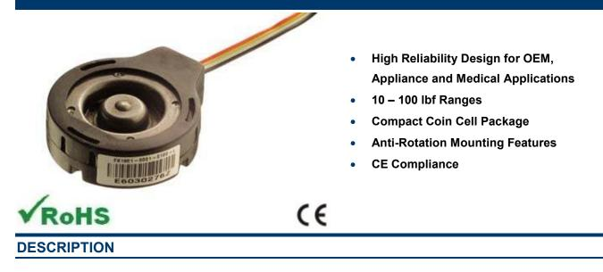
The FX1901 units are intended for OEM use in laboratory, hospital or consumer product applications, establishing a breakthrough price/performance value for compression load cells. The FX1901 is a 1% load cell device with full scale ranges of 10, 25, 50 or 100lbf compression. This new, low-cost technology enables force sensing in a whole new class of "smart" consumer and medical products.
