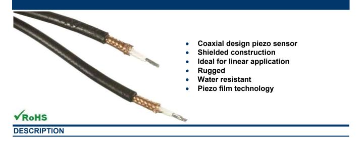
Piezo cable is another form of piezo polymer sensors. Designed as a coaxial cable, the Piezo polymer is the dielectric between the center core and the outer braid. When the cable is compressed or stretched, a charge or voltage is generated proportional to the stress.
