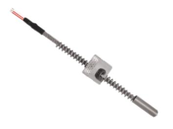
The Extrusion RTD Probe—Bayonet is a miniature, tip sensitive sensor that is used in a wide variety of industries. The sensor is an economical way to spring load a sensor. The spring length and tension can be adjusted as required. The sensors come standard with a spring loaded bayonet fitting. The bayonet fitting keeps the sensitive portion of the sensor engaged with the process while also providing easy removal of the sensor if necessary.
