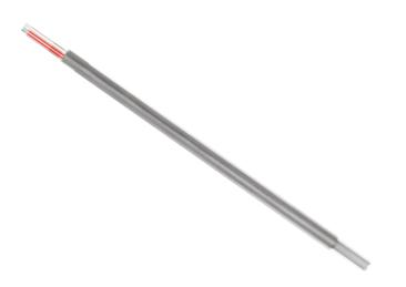
The **Point Sensing RTD Probe** is constructed with a rigid stainless steel sheath with an element embedded into an aluminum tip. The aluminum tip provides faster time response. These sensors are typically designed for use in plenums and ducts within HVAC systems. They can also be utilized whenever a quick time response in a non-corrosive low pressured environment is needed.
