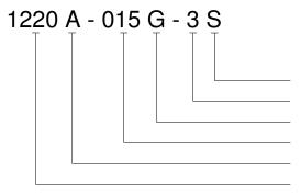
Pressure Tubes (L = Long, S = Short, N = None) Lead Configuration (1,3 - See Dimensions Diagram) Type (G= Gage, A = Absolute, D = Differential) Pressure Range Grade Model
